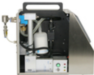
Figure 3: XRC integrated into U-SMPS / DEMC control unit
